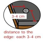
fasten mat (lying on floor) onto the wooden board (low-stress installation)
